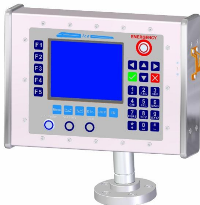
Figure 2: HMI – The communications interface for the driver
